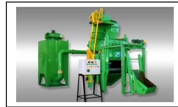
For heavy components Table type machine is preferred. This machine is also designed in different load carrying capacities and size of job. The machine is having various diameter of table like 750mm, 900mm, 1200mm, 1800mm & 2440mm and higher capacities.
