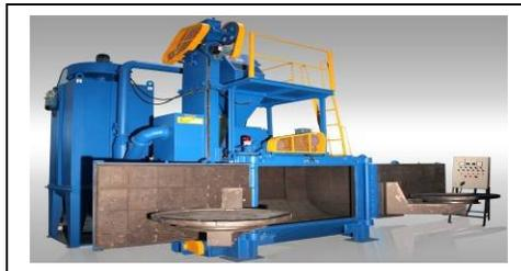
For cleaning of heavy and intricate, hangable forgings and casting the Hanger type machine is now a day preferred. These machines are designed as per customers requirement based on size of forging/casting and output requirement. The following machines are normally preferred.
